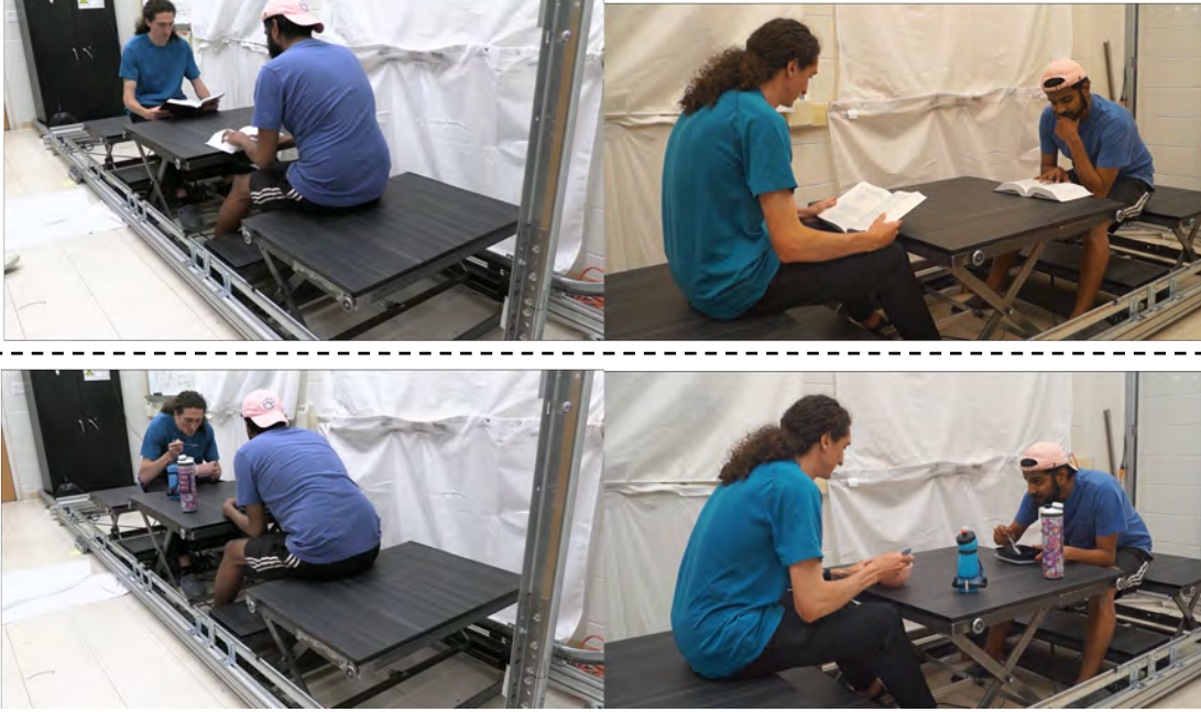
Figure 3.2: Robot system in the ‘table and chair(s)’ configuration supporting a pair of domestic activities, namely, working (top) and eating dinner (bottom).
