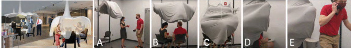
Figure 1.4: Left: A rendering of the robot surfaces elevated and curved downward when people are not seated and seated respectively in the open-plan hotel lobby design case. Right: The full-scale prototype: Two people meet (A) and seat themselves (B), at which point the surface descends and curves (C), “Fully Actuated.” After some time, a member of the party needs to excuse himself for a phone call; the surface “Opens to the Right” (D to E). [16]
