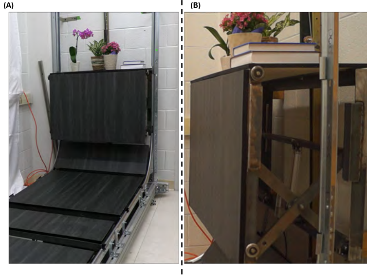
Figure 3.4: Robot system in the shelf configuration, Left; (A) front profile; Right; (B) Side profile.
